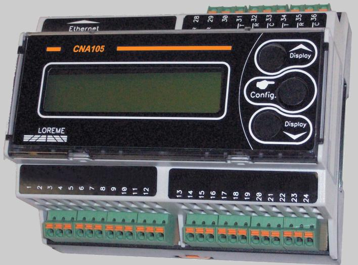
The CNA105 is a converter for parallel outputs encoders. It converts the encoder's position into an analogical signal output. The display allows a quick diagnosis on the proper operation. The CNA105 may be used in many application through its user programmable configuration (encoder resolution, code format type: BCD, gray, binary, polarity, sign, ...).
